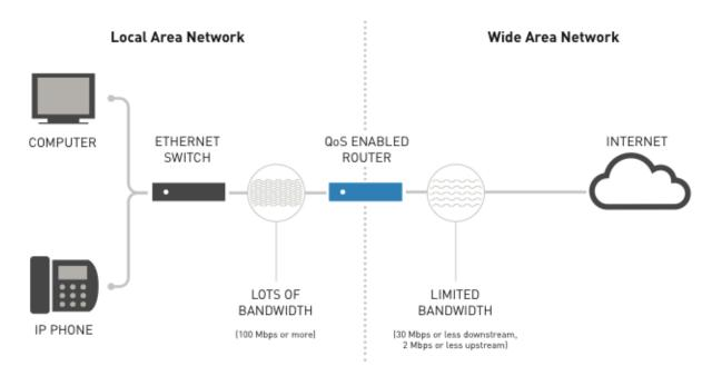
As the diagram above illustrates, a customer network typically has a considerable available bandwidth on the customer premise side (Local Area Network, or LAN) of the
